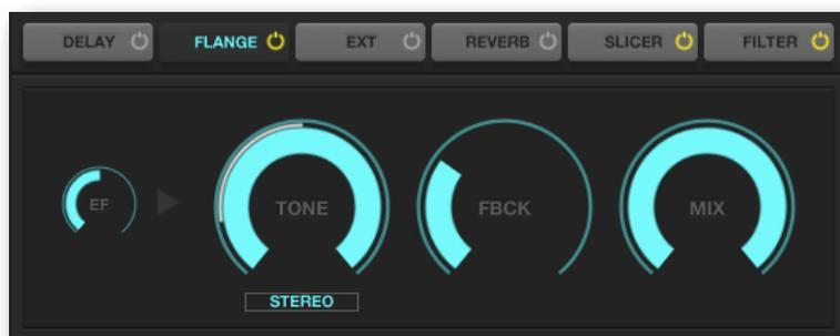
This knob controls the amount and polarity of the envelope signal being routed to the Tone control.
